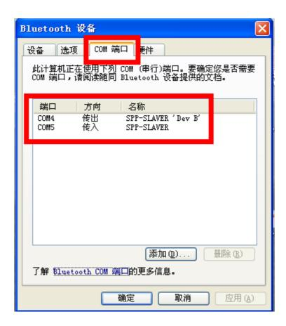
Step 13. Since Bluetooth is direction communication, here we choose COM4, signal comes out to GPRINTER. Go back to GP-80160IIN Property dialog box, choose COM4 serial port and Apply.
